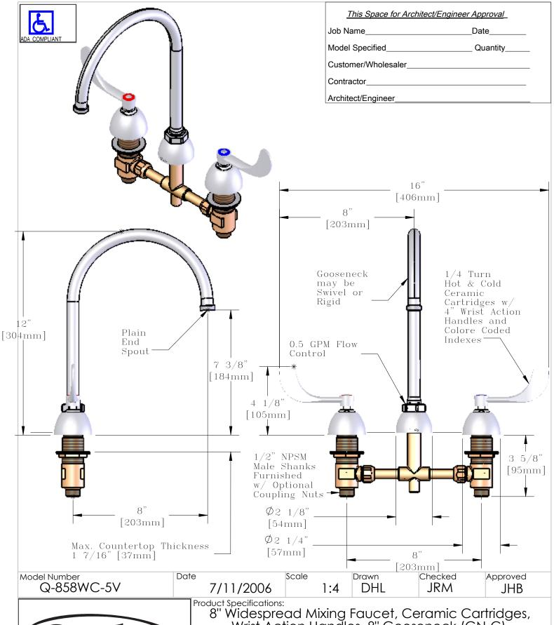
8" Widespread Mixing Faucet, Ceramic Cartridges, Wrist Action Handles, 8" Gooseneck (GN-C), 0.5 GPM Flow Control
