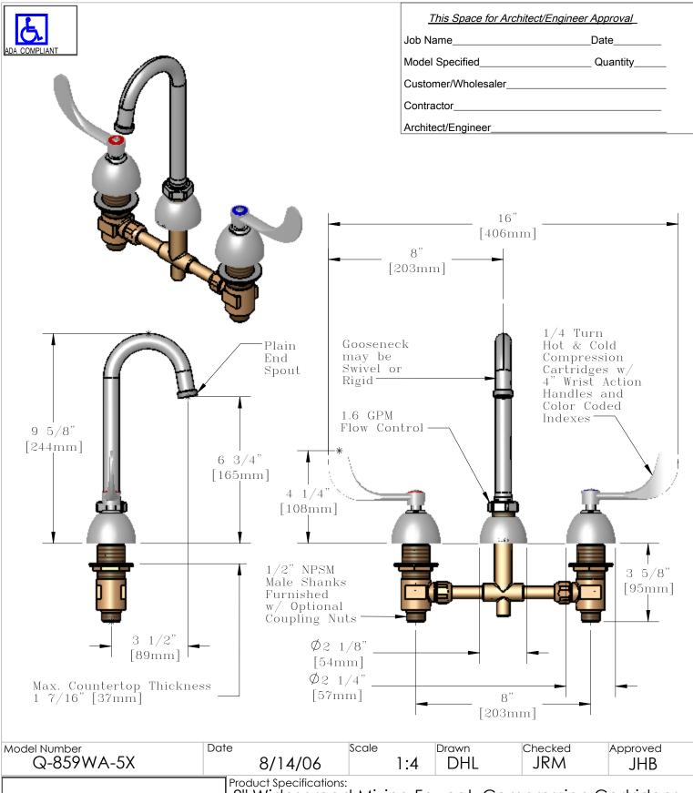
8" Widespread Mixing Faucet, Compression Cartridges, Wrist Action Handles, 3 1/2" Gooseneck (GN-A), 1.6 GPM Flow Control
