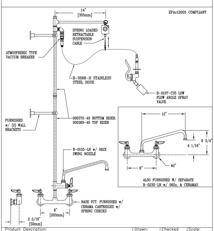
8" c/c Wall Mount Base Faucet, Add-on-Faucet, 12" Swing Nozzle, Horizontal Balancing Arm, Retractable Cable, 68" Flex. Hose w/ Angle Spray
