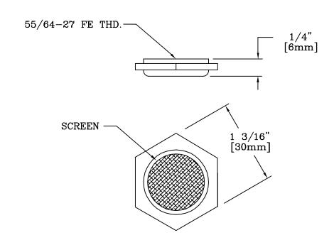
NOTE: EPOXY CEMENTED ON NOZZLES & GOOSENECKS WHEN FURNISHED ON ORIGINAL EQUIPMENT.
