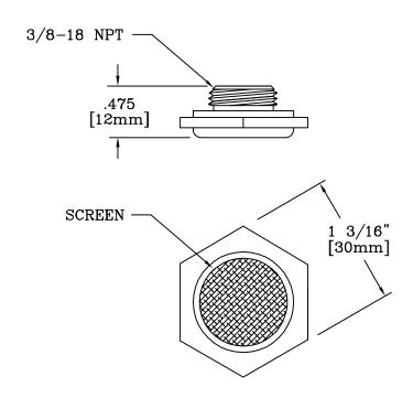
NOTE: EPOXY CEMENTED ON NOZZLES & GOOSENECKS WHEN FURNISHED ON ORIGINAL EQUIPMENT.
