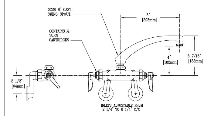
FURNISHED w/ (2) 007x WASHERS TO CONVERT SWIVEL to RIGID. TO INSTALL: UNSCREW NOZZLE, LIFT OUT, & PLACE WASHERS IN SWIVEL BODY. THEN RE-INSTALL NOZZLE
