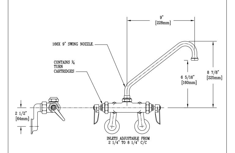
FURNISHED w/ (2) 007x WASHERS TO CONVERT SWING NOZZLE to RIGID. TO INSTALL: UNSCREW NOZZLE, LIFT OUT, & PLACE WASHERS IN SWIVEL BODY. THEN RE-INSTALL NOZZLE
