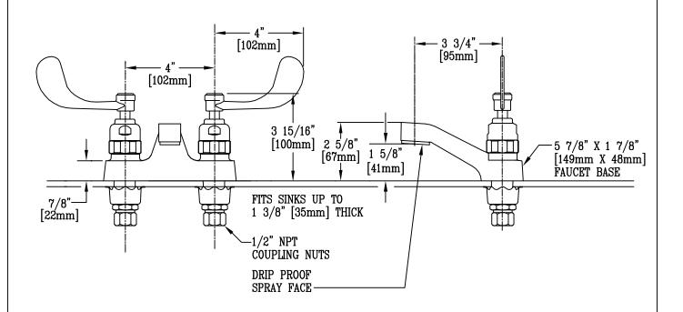
FLOW ADJUSTABLE FROM INSTANTANEOUS SHUTOFF TO EXTENDED FLOW
