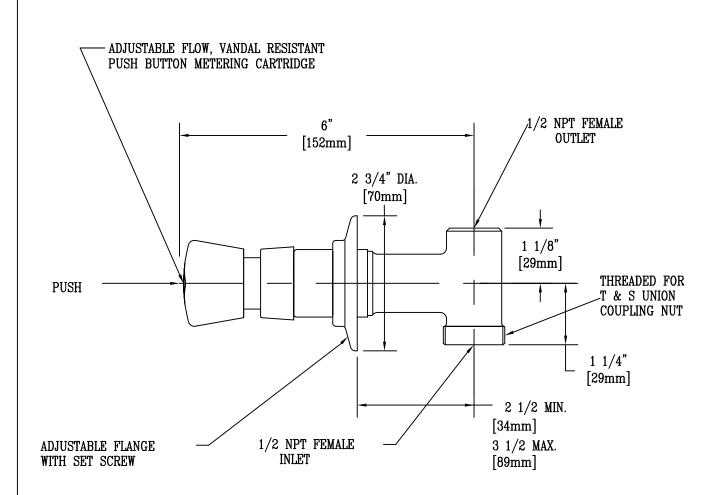
ADD - UCP SUFFIX FOR 1/2 IPS FEMALE UNION INLET ADD - UCT SUFFIX FOR 5/8 0.D. COPPER TUBING
