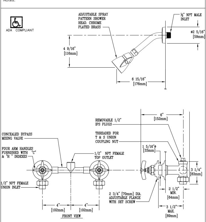
Product Description: CONCEALED BYPASS MIXING VALVE WITH B-1060 1/2" NPT FEMALE INLETS & OUTLET, FOUR ARM HANDLES & ADJUSTABKE SHOWER HEAD
