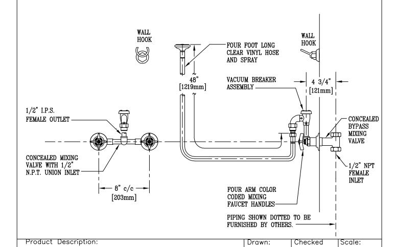
CONCEALED MIXING VALVE & BED PAN WASHER
