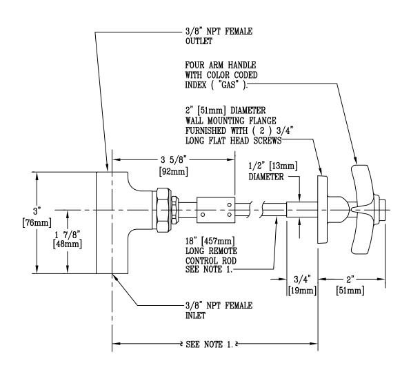
NOTE 1: STANDARD ROD LENGTH IS 18". WHEN ORDERING, SPECIFY ACTUAL LENGTH DESIRED. MINIMUM IS 4 1/2" [114mm]
