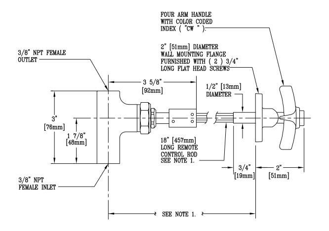
NOTE 1: STANDARD ROD LENGTH IS 18". WHEN ORDERING, SPECIFY ACTUAL LENGTH DESIRED. MINIMUM IS 4 1/2" [114mm]
