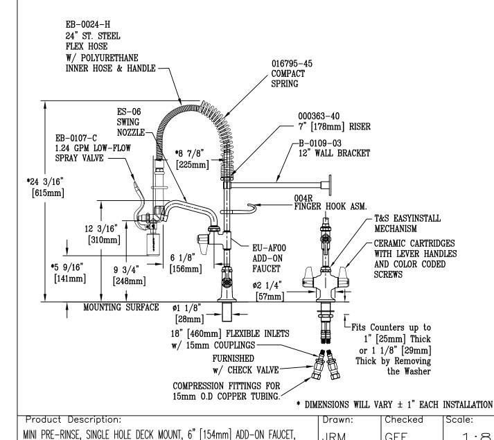
LOW-FLOW SPRAY VALVE, 12" [305mm] WALL BRACKET, 18" FLEX
