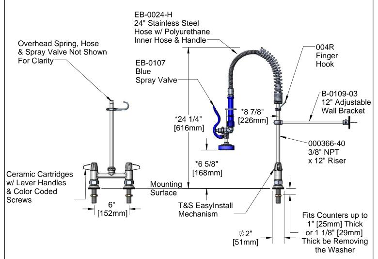
Note: Rough-In Requirements ∅1" [25mm] Holes at 6" [152mm] c/c
